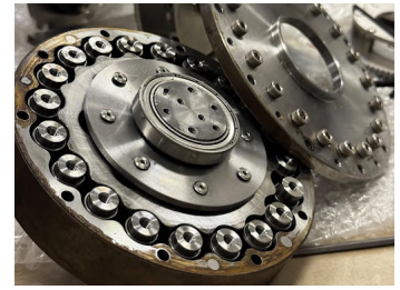
(a) Details of the Arm7.0 link lengths. (b) Lateral movement mechanism. (c) Developed cycloidal reducer.
