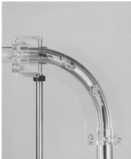
Fig. 14 Locomotion through a vertical elbow-joint
