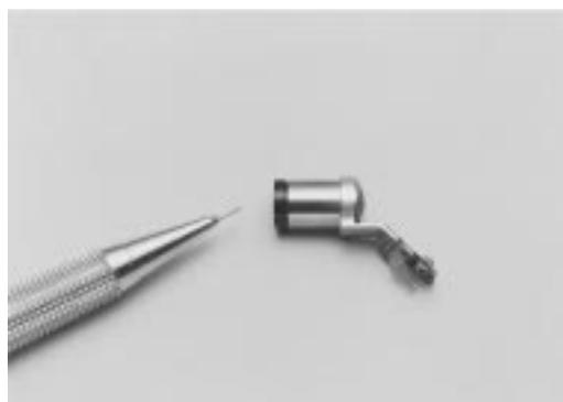
Fig. 8 The outline of micro CCD camera head
