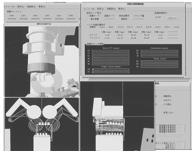
Fig. 13 Example of CG display (Solid model:predictive display, Wireframe: Virtual camera, Upper right; Multisensor bargraph)
