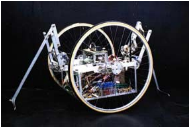
Fig.2: Leg-wheel robot Chariot . The radius of the wheel is 32cm and the length of the leg is 85cm when expanded. The weight of Chariot is about 20Kg.
